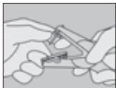
Figure 1 Disinfect pliers prior to use. Place male button onto pin until it projects through the tip.
